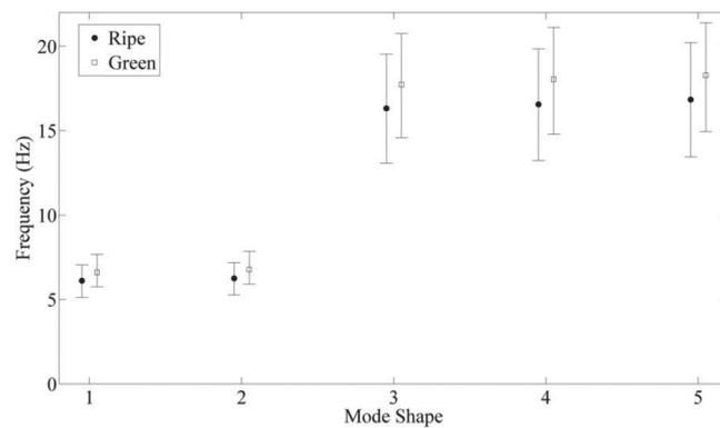
FIGURE 7 - Natural frequencies for the branch as obtained in this work and by Filgueiras (2001).
