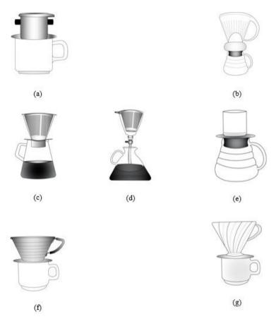
**FIGURE 1 -** Gravity-drip filtration coffee preparation methods a) Vietnamese, b) Clever, c) Kinto, d) Yama, e) RS 16, f) V60 Kalita, and g) V60. Source: Author elaboration.
